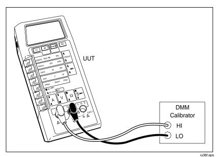
Figure 5-5. Equipment Connection for Current Test
