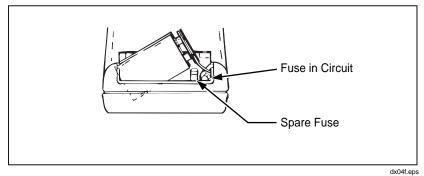
Figure 2-2. Battery Removal and Fuses
