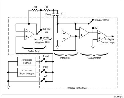
Figure 4-2. Analog Portion of the A/D Converter
