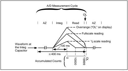
Figure 4-3. A/D Measurement Cycle
