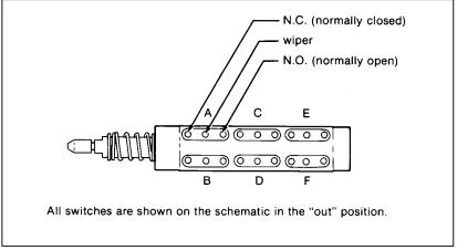
Figure 7-4. Switch Detail
