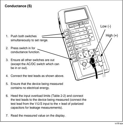
Figure 2-14. Conductance Operation
