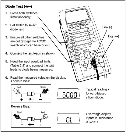
Figure 2-16. Diode Test
