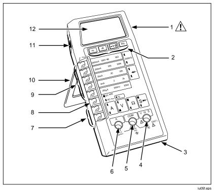
Figure 2-3. Controls, Indicators and Connectors
