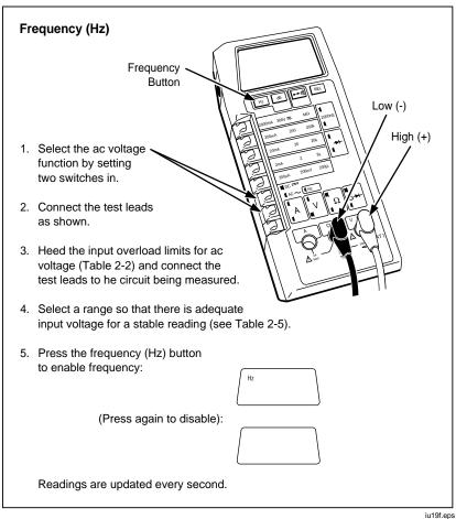
Figure 2-18. Frequency (Hz) Operation
