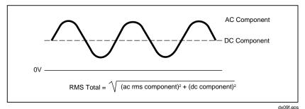
Figure 2-7. AC and DC Waveform Components
