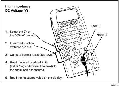
Figure 2-9. High Impedance DC Voltage
