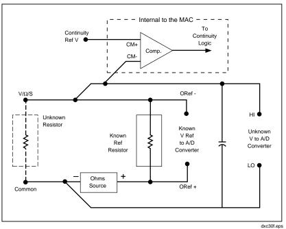
Figure 4-6. Resistance/Conductance/Continuity Measurement
