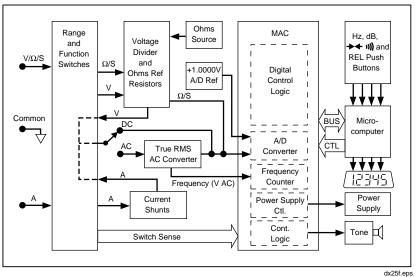
Figure 4-1. 8060A Block Diagram
