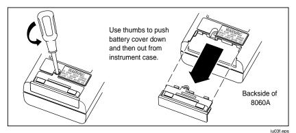
Figure 2-1. Removal of Battery Compartment Cover
