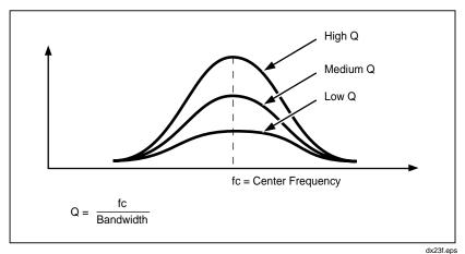
Figure 3-2. Measuring Q with the 8060A
