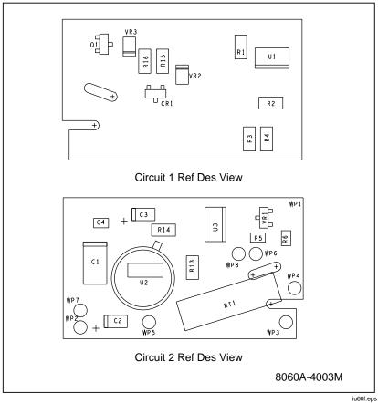
Figure 6-3. A3 Rms PCB Assembly
