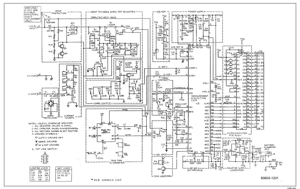
Figure 7-5. A1 Main PCB Schematic Diagram
