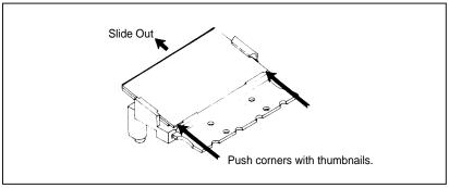
Figure 5-3. Disassembling the LCD
