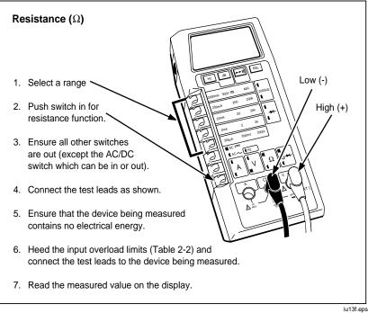
Figure 2-12. Resistance Operation
