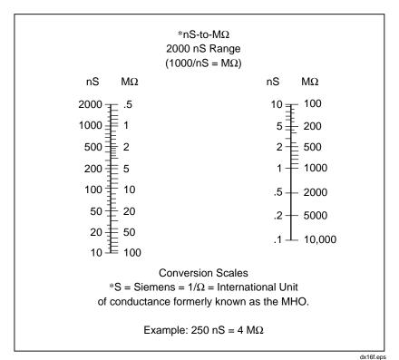
Figure 2-15. Conductance/Resistance Conversion
