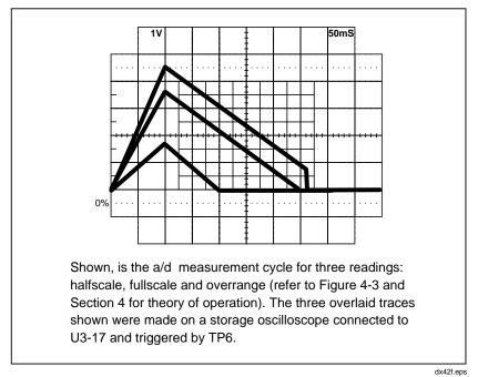
Figure 7-3. A/D Measurement Cycle
