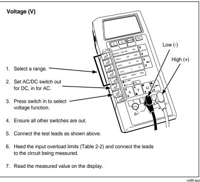
Figure 2-6. Voltage Operation
