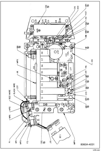
Figure 7-1. A1 Main PCB Component Locations
