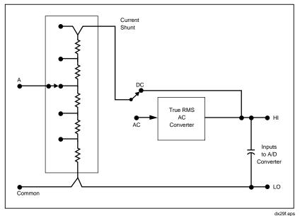
Figure 4-5. Current Measurement
