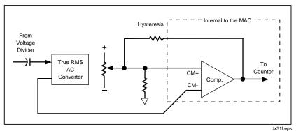
Figure 4-7. Frequency Measurement
