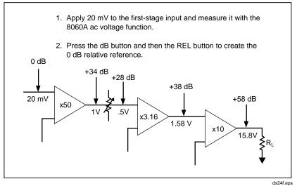
Figure 3-3. Measuring Stage Gain with Relative dB
