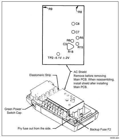
Figure 5-1. Calibration and Backup Fuse (F2) Access)
