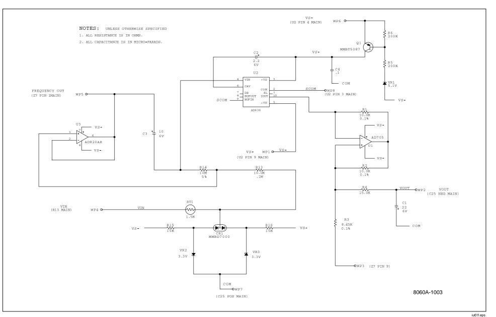
Figure 7-6. A3 Rms PCB Schematic Diagram
